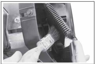
Figure 18. Cleaning Underside of Oil Cooler.
