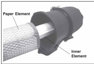
Figure 21. Removing Elements.
