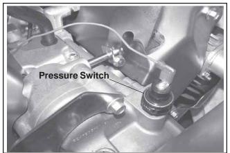
Figure 11. Oil Sentry<sub>™</sub> Pressure Switch.
