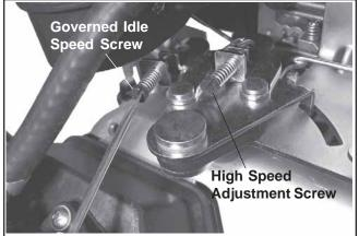
Figure 27. Adjusting Governed Idle Speed Screw.
