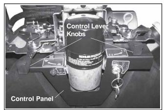
Figure 8. Optional Control Panel with Engine Mounted Controls.
