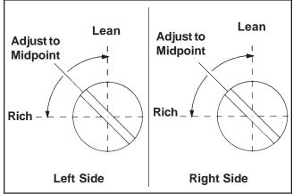
Figure 28. Optimum Low Idle Fuel Settings.
