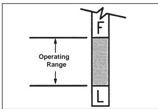
Figure 10. Oil Level Marks on Dipstick.
