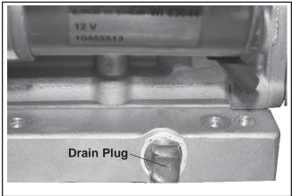
Figure 12. Oil Drain Plug (Starter Side).
