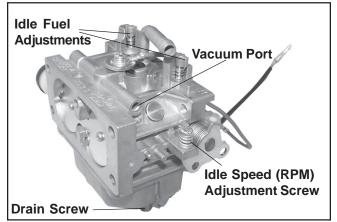
Figure 26. Keihin Two-Barrel Carburetor.
