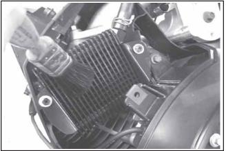
Figure 17. Cleaning Top of Oil Cooler.
